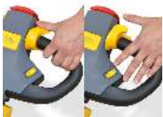
Automatic braking system when operator releases the throttle
